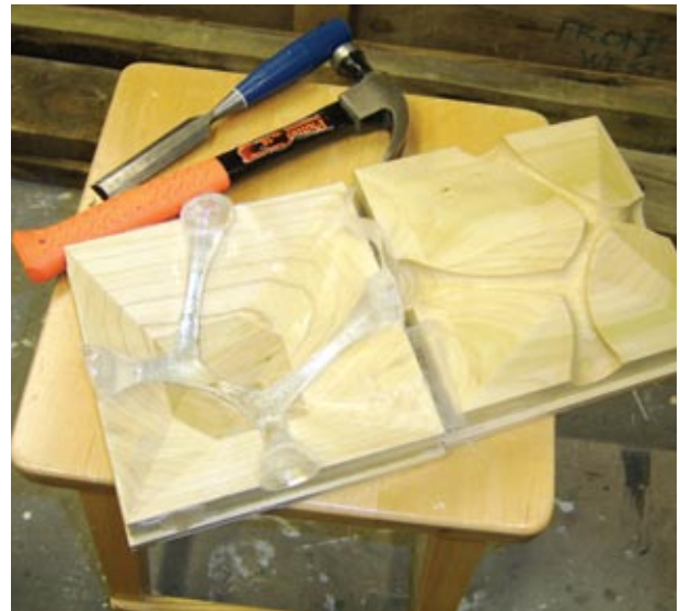
Figure 19: Final casting is opened after curing process.
