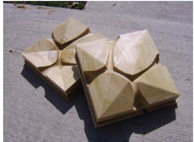
Figure 18: Final machined poplar mold with lacquer finish for mold removal.
